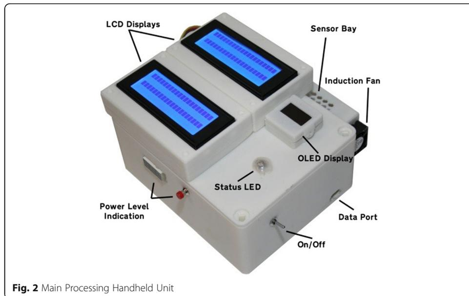
environmental sensors and includes an induction fan to ensure that adequate sampling of ambient air is constantly being monitored. The user interface is comprised of a set of two LCD displays and an OLED display and a Status LED. The three displays are used to provide the learner with training information based on the context and location of the device. The status LED is used to warn the learner of potential patient threats obtained from the location of the device.
