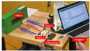
Fig. 3 One of the mini-project-based homework assignments: ultrasonic sensor calibration
