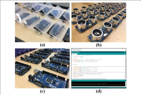
**Fig. 2** Hardware and software for mini-project-based homework assignments. **a** Robotics development kit. **b** Ultrasonic sensors. **c** Arduino development board. **d** Arduino integrated development environment
